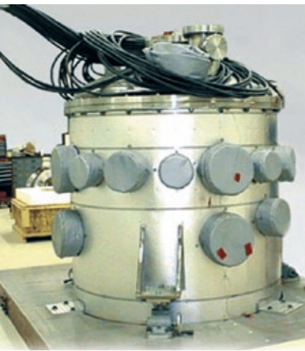
FIGURE 8 Picture of the Sustained Spheromak Physics Experiment (SSPX) apparatus. Plasma and magnetic fields are created in a toroidal arrangement within this structure. Source: David Hill, Lawrence Livermore National Laboratories.
